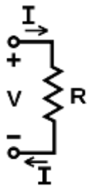
Figure 1: V (voltage), I (current), and R (resistance), the parameters of Ohm's law.
